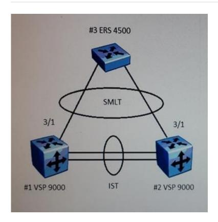
Simple Loop Prevention Protocol (SLPP) provides active protection against Layer 2 network loops on a per-VLAN basis. For the SLPP Tx process, the network administrator decides on which VLANs to enable SLPP. The hello packets are then replicated out all ports that are members of the SLPP-enabled VLAN.
