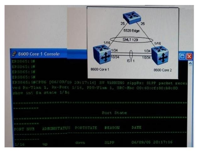
A technician has just enabled SLPP on both core switches, and is reviewing the network diagram and console output from the core 1 Ethernet Routing Switch (ERS) 8000.
