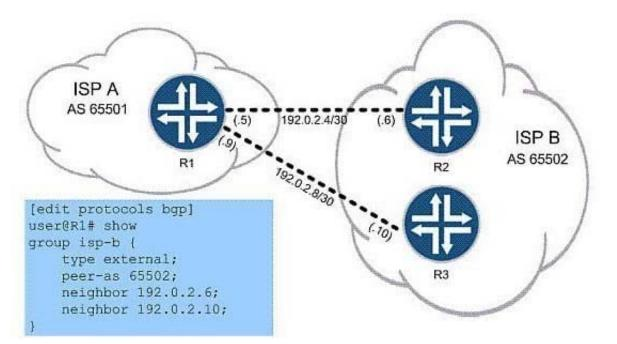
Referring to the exhibit, you work for ISP A and are asked to configure R1 to forward traffic for all routes across both available links, to both routers in ISP B\\'s network. Which three configuration commands do you use? (Choose three.)
