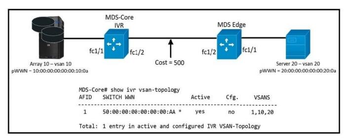
An engineer is configuring Inter-VSAN routing for two Cisco MDS switches. The FSPF cost between the switches is 500, and the Cisco MDS core virtualizes an IVR NAT domain as shown. Which statement about the topology is correct?
