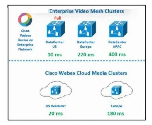
Refer to the exhibit. A Cisco Webex device on an enterprise network has identified the given STUN round-trip delays in milliseconds to the enterprise Video Mesh clusters and two Webex Cloud Media clusters during the call setup. Which correct sequence of clusters is the client connecting to?
