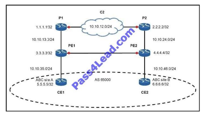
An engineer is looking the CE1 routing table for CE2 Loopback 0. Each CE runs OSPF with its PE.
