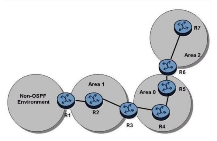
In the topology shown, router R1 is an ASBR configured to export external routes to OSPF. Assuming that there are no stub networks, which of the following statements regarding Type 4 LSA generation is true?
