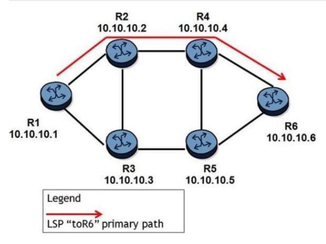
An LSP traverses R1-R2-R4-R6 and facility fast reroute with link protection is enabled. All links have the same cost. Which of the following about PLRs and MPs is TRUE?
