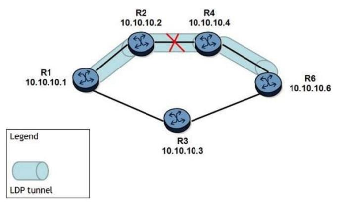
An LDP tunnel is established on router R1 towards router R6. The link between routers R2 and R4 goes down. What will happen to the MPLS data traffic to router R6 IMMEDIATELY after the link goes down?
