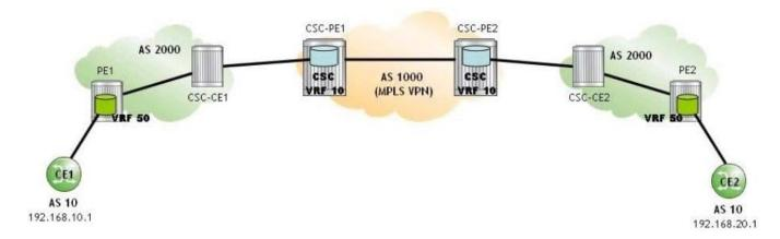
A Carrier Supporting Carrier (CSC) VPRN is configured for a customer carrier who is a BGP/MPLS service provider. Which of the following describes the routes present in PE1\\'s global routing table?
