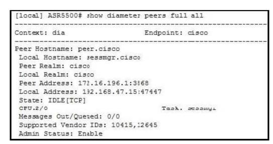
The locally configured Diameter peer does not seem to be communicating with its remote peer. Which option describes the problem?
