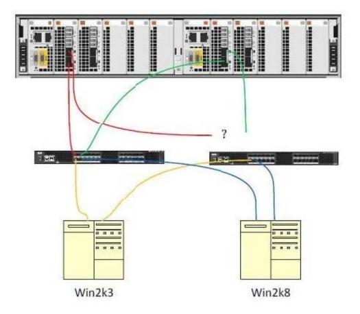
A customer has a two-fabric SAN with hosts and a single CX4-480 cabled redundantly to both switches. SPA port 0 is plugged in to port 0 of Switch A. According to EMC best practice, which SP port should be plugged in to port 0 of Switch B?
