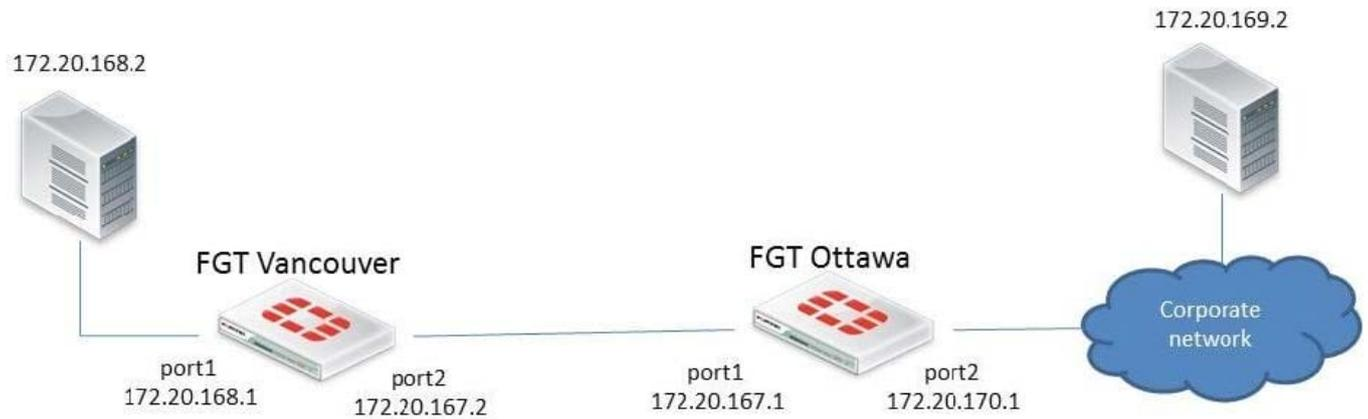
In this scenario, the Fortigate unit in Ottawa has the following routing table: S\* 0.0.0.0/0 [10/0] via 172.20.170.254, port2 C 172.20.167.0/24 is directly connected, port1 C 172.20.170.0/24 is directly connected, port2
