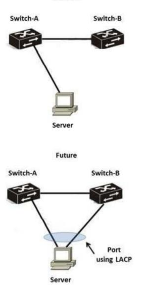
A network administrator has a server with a single link to the network. The company is concerned about redundancy and wants to implement a solution like that shown in the right-hand side of the diagram.
