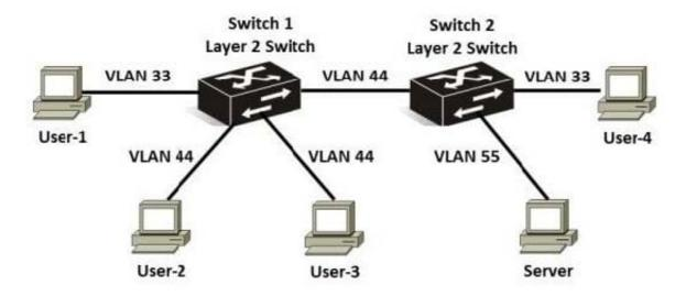
Switch 1 and Switch 2 are HP ProVision switches operating as Layer 2 switches. VLAN 33 has been defined as the management VLAN on both switches. Based on this topology, which user devices can access Switch 1 by using SSH?
