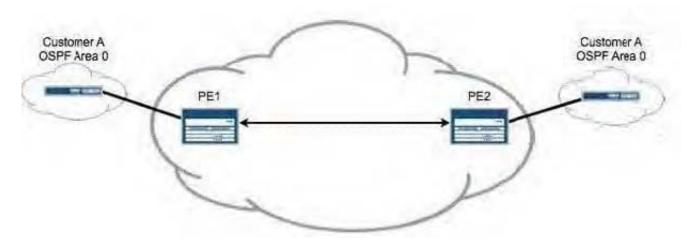
Referring to the exhibit, Customer A is complaining that no OSPF routes are being received across your Layer 3 VPN. You suspect that a problem exists with the PE-CE protocol. The core network is operational. Which operational command on PE1 helps troubleshoot this problem?
