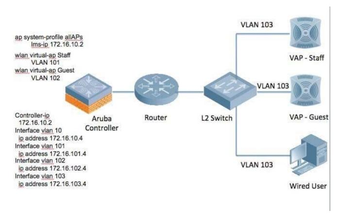
In the above diagram, the system shows two Aruba access points. Which VLANs must be configured on trunk link D between the router and Aruba controller to support wireless users when the controller is provisioned for L2 operations?
