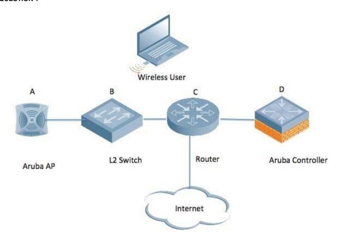
In the diagram provided for this question, the wireless user\\'s laptop is associated with an Aruba AP in tunnel forwarding mode. The AP terminates on the local controller.
