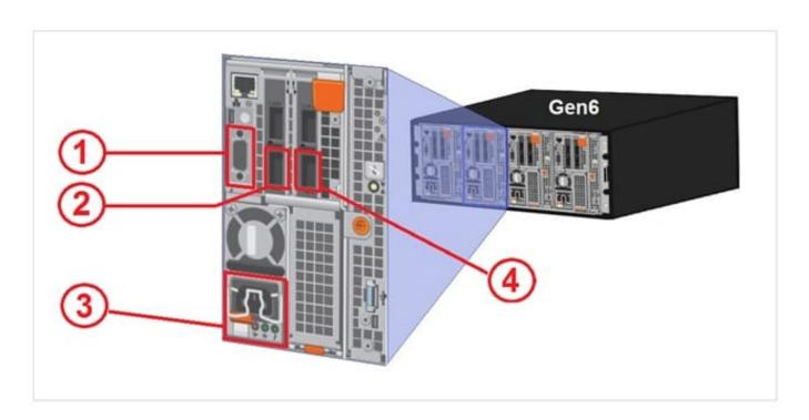
In an Isilon environment, match the connectivity type to the proper numerical port reference shown in the exhibit.
