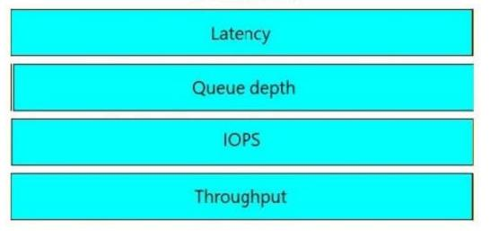
Throughput = Sized by type and number of ports to handle traffic Latency = Time taken for an IO to be executed IOPS = Amount IO generated by application Queue depth = IOS in buffer waiting to be executed
