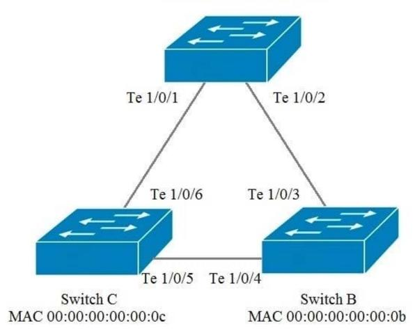
The exhibit represents a topology with all Dell EMC N4000 Series switches with RSTP enabled. In addition, the switches are using the default configuration on all ports and protocols. Which port number will be blocked by spanning tree?
