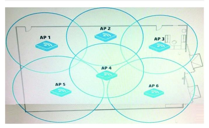
A company has many dual-radio APs that are deployed relatively closely together. They are controlled by an HP Unified Wired-Wireless controller. The administrator wants to implement load balancing among the radios on different APs.
