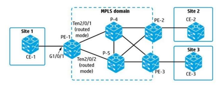
An administrator is configuring an MPLS VPLS Martini solution on PE-1. The VPLS solution should connect customer A sites 1, 2, and 3 Where should the administrator specify the LDP peers and pseudo wire (PW) label for the PWs?
