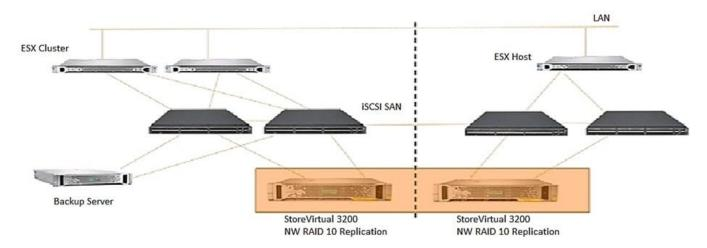
An HPE StoreVirtual 3200 system consists of 19x 1.2 TB Drives in a RAID5 with a capacity level of 75%. The network is built with four HPE FlexFabric 5900 switches. The customer complained about performance challenges with the given configuration, and the administrator identified the drive configuration as a bottleneck. A performance analysis shows latencies above 60ms. Installation of the systems was done by best practices.
