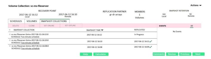
A customer with an existing HPE Nimble installation sends you the output shown. The administrator who initially set up the replication has left the company. They ask you what the current RPO level for their replication is. How should you respond?
