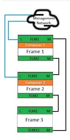
You are installing three Synergy frames for a customer PoC in the configuration shown. The composer is unable to discover the frames.
