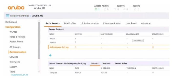
You have set up a RADIUS server on an ArubaOS Mobility Controller (MC) when you created a WLAN named "MyEmployees . You now want to enable the MC to accept change of authorization (CoA) messages from this server for wireless sessions on this WLAN.
