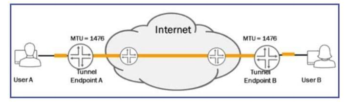
You have created a GRE tunnel as shown in the exhibit. The router with tunnel endpoint A is dropping the packets originating from User A and destined to User B.
