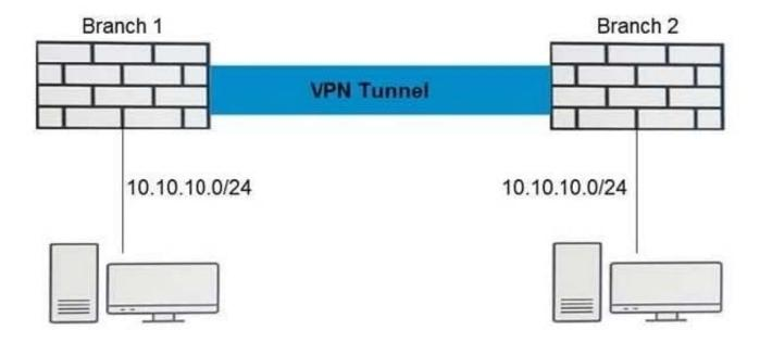
Branch 1 and Branch 2 have an active VPN tunnel configured, but internal hosts cannot communicate with each other.
