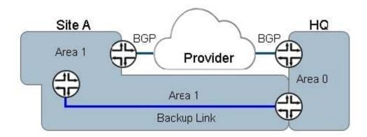
Site HQ connects to Site A through a provider using BGP. The BGP route for Site A destinations is redistributed info OSPF within site HQ. You provision a backup link over a dedicated leased line that connects to Site A, which should only be used when Site A is not reachable through the provider.
