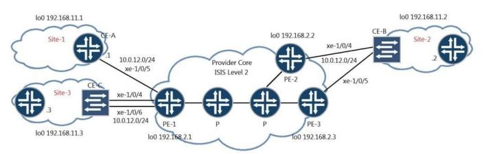
You have the LDP signaled VPLS topology as shown in the exhibit. CE-B at Site-2 is multihomed to both PE-2 and PE-3.
