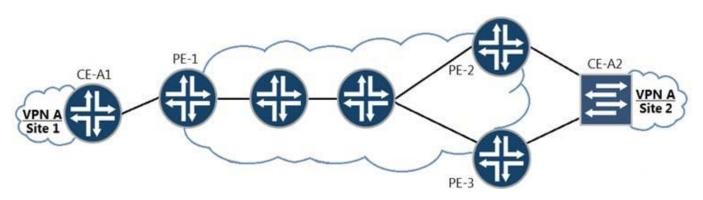
Referring to the exhibit, you need to implement VPLS between CE-A1 and CE-A2. You must ensure that no loops are created due to the multihoming of the connection from CE-A2 to PE2 and PE3.
