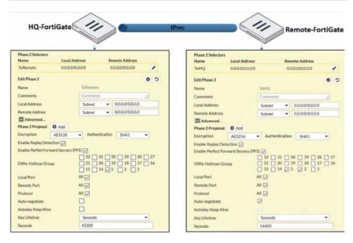
A network administrator is troubleshooting an IPsec tunnel between two FortiGate devices. The administrator has determined that phase 1 status is up. but phase 2 fails to come up.
