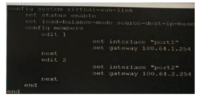
Based on the exhibit, which algorithm does SD-WAN use to distribute traffic that does not match any of the SD-WAN rules, among the member interfaces?
