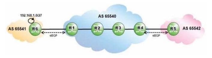
AS 65540 is using MPLS to provide BGP shortcuts for its iBGP routing. Which routers must be configured with the "configure router bgp igp-shortcuts rsvp-te" command?
