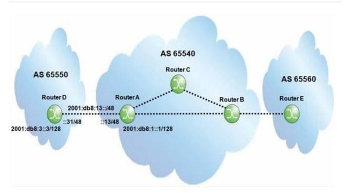
Assume all router-IDs are properly configured. Which of the following configurations is required on the Alcatel-Lucent 7750 SR router A to establish an IPv6 BGP session to router D?
