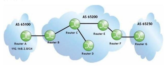
Routers C and E are route reflectors. When the update for prefix 192.168.2.0/24 is received at router F, what will be the Originator\_ID attribute?
