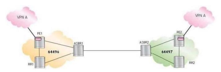
Routers RR1 and RR2 are configured as route reflectors. For the inter-AS model C VPRN, which of the following about the BGP sessions established between the routers is TRUE?
