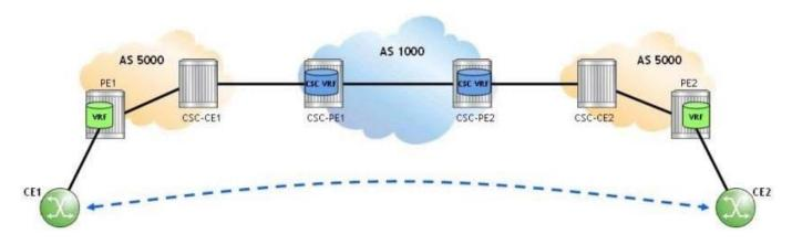
A Carrier Supporting Carrier (CSC) VPRN is configured on an Alcatel-Lucent 7750 SR for a customer carrier offering VPRN services. Which of the following about this configuration is FALSE?
