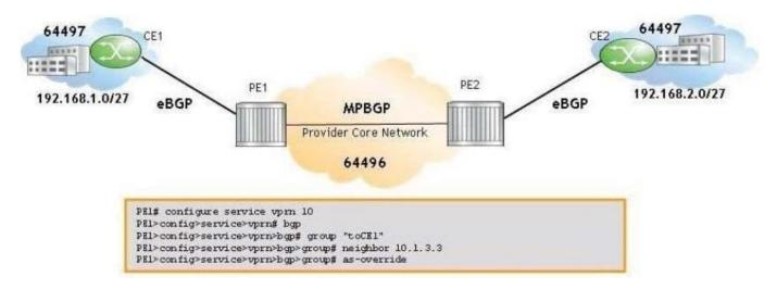
AS-override is configured on PE1 to eliminate the BGP loops. What is the expected AS-Path in the VPNIPv4 route 64496:10:192.168.2.0/27 received by PE1?
