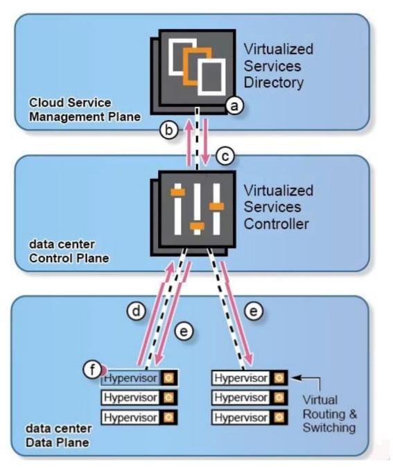
What is the correct sequence of events for a VM to be instantiated, and for its required network connectivity to be created with the Nuage VCS solution?
