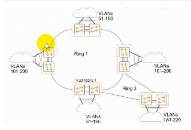
which shows the topology tot an Ethernet Ring Protection Switching (ERPS) solution.
