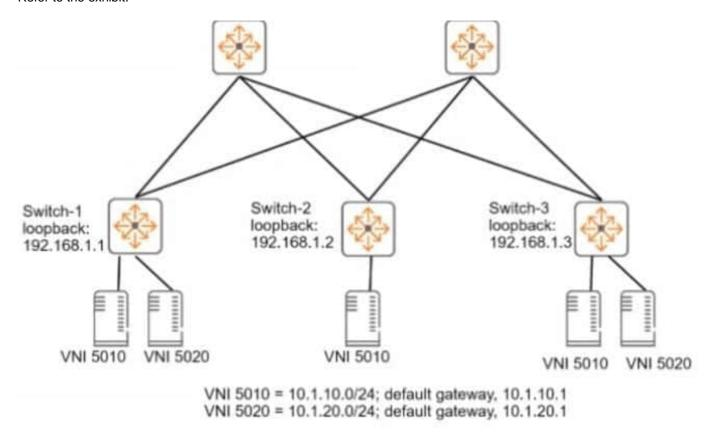
You need to set up an ArubaOS-CX switch to implement Virtual Extensible LAN (VXLAN) WITHOUT Ethernet VPN (EVPN). The exhibit Indicates which servers should be part of the same VXLANs and the desired VNIs for the VXLANs. Assume that the network is already configured to permit each ArubaOS-CX switch to reach each other switch\\'s loopback interface.
