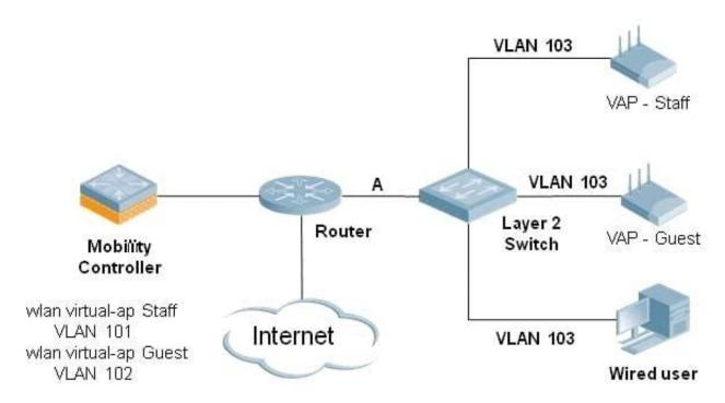
In the above diagram, the system shows two Aruba access points and a wired user.
