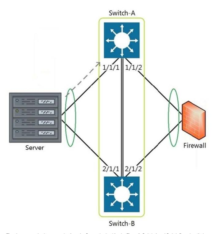
The above scenario shows a packet from the Server destined for the Firewall. Switch-A and Switch-B are bundled as VSF stack. The LAG between the VSF stack and the firewall indicates a hash function to forward the packet on port 2/1/2. Which statement is true regarding how Switch-A will forward the packet?
